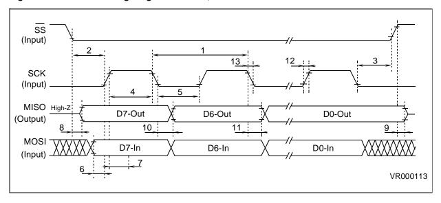
Figure 47. SPI Slave Timing Diagram CPOL=1, CPHA=0
