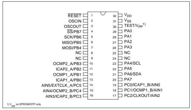
Figure 3. ST72251 Pinout (SO28)
