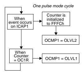
Then, on a valid event on the ICAP1 pin, the counter is initialized to FFFCh and OLVL2 bit is loaded on the OCMP1 pin. When the value of the counter is equal to the value of the contents of the OC1R register, the OLVL1 bit is output on the OCMP1 pin, (See Figure 25).
