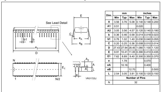
Figure 50. 32-Pin Shrink Ceramic Dual In-Line Package
