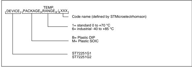
Figure 52. OTP User Programmable Device Types
