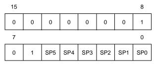
The Stack Pointer is a 16-bit register which is always pointing to the next free location in the stack. It is then decremented after data has been pushed onto the stack and incremented before data is popped from the stack (see Figure 6).
