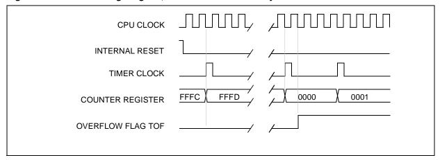
Figure 20. Counter Timing Diagram, internal clock divided by 8
