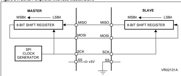
Figure 32. Serial Peripheral Interface Block Diagram
